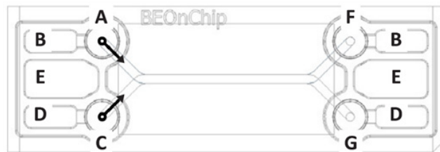
Figure 2. Top view of BE-Doubleflow chip: A) Upper channel inlet and inlet reservoir, B) upper channel medium overflow reservoir, C) bottom channel inlet and inlet reservoir, D) bottom channel medium overflow reservoir, E) evaporation reservoir, F) upper channel outlet and outlet reservoir, G) bottom channel outlet and outlet reservoir. Modified from BE-Doubleflow technical characteristics data sheet.
