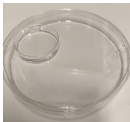
Figure 3. Humidity chamber made with petri dishes for BE-Doubleflow chips.
