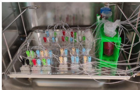
Figure 4. BE-Doubleflow chips connected to a pump in a humidified incubator.
